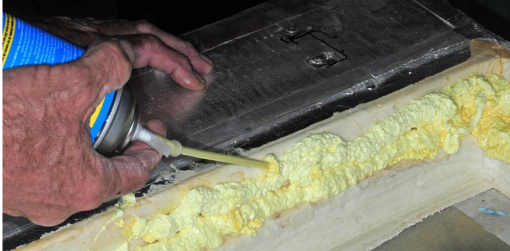
Two beads of liquid foam are applied to the foam pack on the refrigerator cabinet. This will seal off any gaps once the new cooling is in place and the foam expands.
