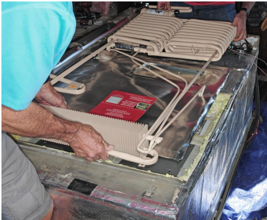
Two beads of liquid foam are applied to the foam pack on the refrigerator cabinet. This will seal off any gaps once the new cooling is in place and the foam expands.
